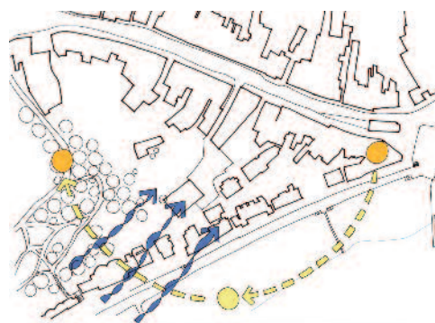
Siting: buildings should be positioned to optimise free aspects of climate, such as sun, wind and topography
