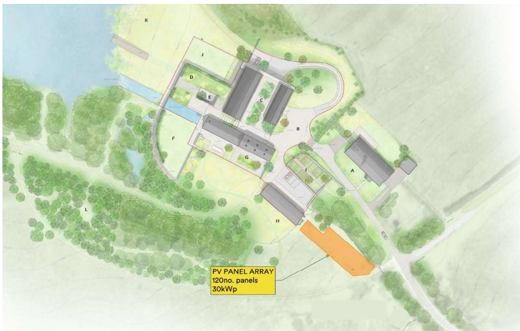
Figure 1- PV array (orange) location
